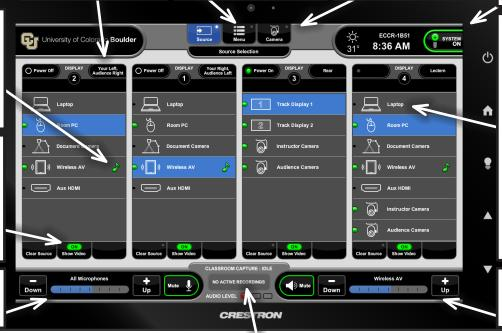
When a device is connected using the provided cables, "Laptop" will automatically be selected on DISPLAY 1 and DISPLAY 2
